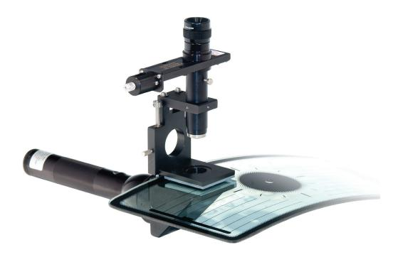
The GES-100 Edge-Stress Meters are light, portable, battery-operated instruments specially designed to measure edge stress in annealed, heat-strengthened, and tempered glass. The procedure is non destructive, and can be used on both flat and curved glass.
